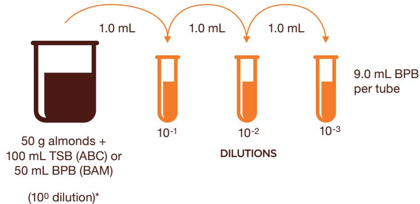
\*ABC Procedure—A correction factor of x2 is needed in calculations for 1:2 w/v dilution
