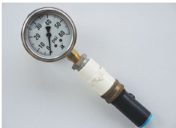
Figure 16. Pressure gauge adapted for measurement at tail end of lateral line microirrigation system tubing. (Photo by L. Schwankl)
