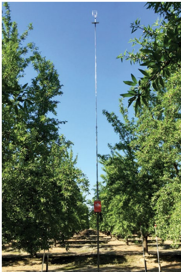
Figure 12. Tule in-field hardware used to collect data for ET estimation. (Photo by tuletechnologies.com )
