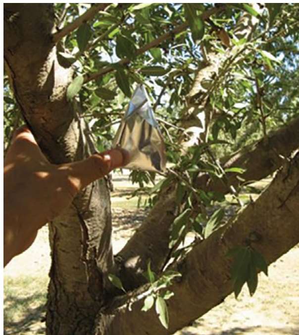
Figure 4. Lower interior leaves are selected on almond trees to measure SWP. (Photo by A. Fulton)
