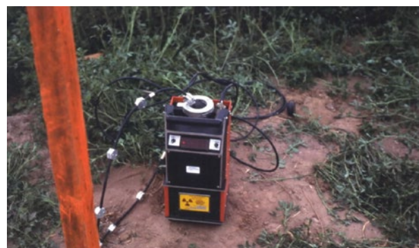
Figure 4. Neutron probe soil moisture meter. (Photo by L. Schwank)
