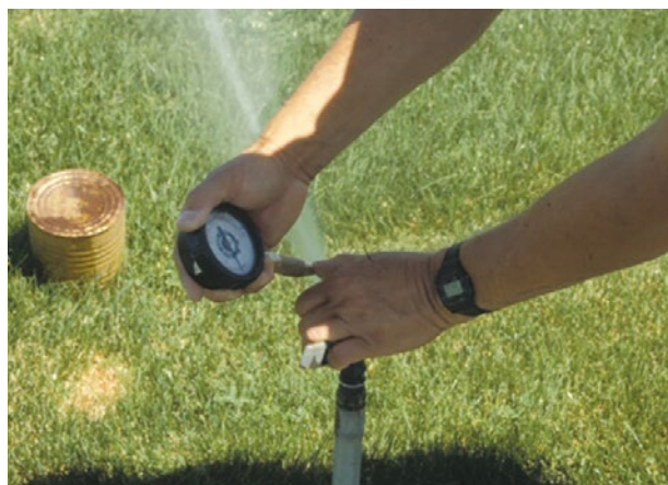
Figure 6. Water pressure is read by positioning the pitot tube directly in the sprinkler's water stream. (Photo by L. Schwankl)
