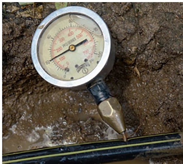
Figure 19. A pitot tube fitted with a pressure gauge adapted for measurement within microirrigation tubing system.
