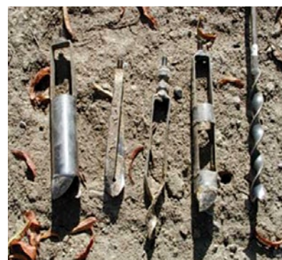
Figure 1. Various types of augers that can be used to sample the soil moisture content. (Photo by B. Sanden)
