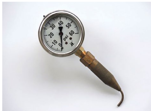
Figure 17. A pitot tube fitted with a pressure gauge adapted for measurement within microirrigation tubing system. (Photo by L. Schwankl)
