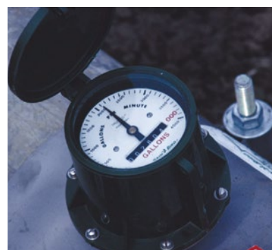
Figure 1. Flow meter register (readout) of a propeller saddle-mount flow meter. Flow meters allow for more accurate and easily obtainable measures of applied water. (Photo by L. Schwankl)
