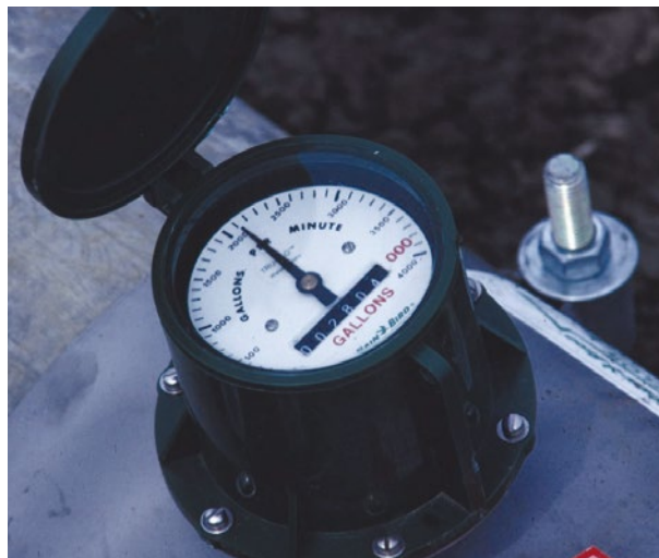
Figure 2. Flow meter register (readout) of a propeller saddle-mount flow meter. Flow meters allow for more accurate and more easily obtainable measures of applied water. (Photo by L. Schwank)
