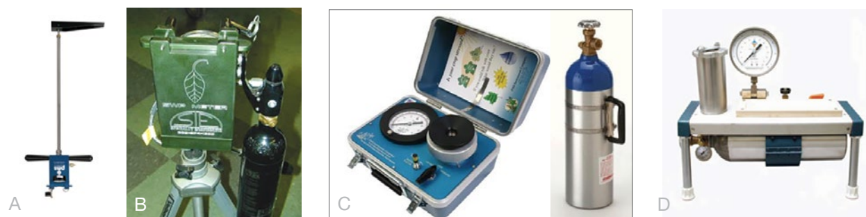
Figure 5. Four examples of commercially available pressure chambers. Example A is a pump-up style by PMS Instruments in which a foot pump creates air pressure in the rectangular chamber. Example B, by Specialty Engineering, also has a rectangular chamber, employs a tripod to hold the pressure chamber, and uses compressed carbon dioxide (CO 2 ) gas to supply the pressure. Example C is a suitcase-style pressure chamber. It has a cylindrical chamber that uses an external source of nitrogen gas, stored in a metal cylinder, to pressurize the chamber. Both PMS Instruments and Soilmoisture Equipment Corp. offer this style of pressure chamber. Example D is a console- or bench-style pressure chamber by Soilmoisture Equipment Corp. that also uses an external bottle of nitrogen gas to pressurize the chamber. Photos: Courtesy of Plant Moisture Stress (PMS) Instrument Company, Albany, OR (A, C); Specialty Engineering, Waterford, CA (B); and Soilmoisture Equipment Corp., Santa Barbara, CA (D).
