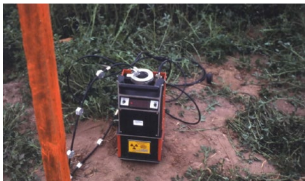
Figure 5. Neutron probe soil moisture meter. (Photo by L. Schwankl)
