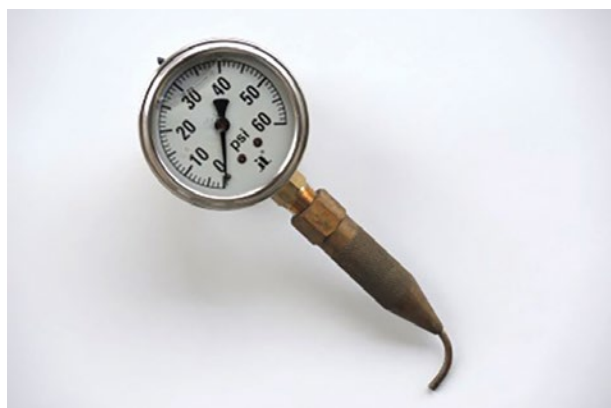
Figure 5. A pitot tube fitted with a pressure gauge works well for taking sprinkler pressure measurements. (Photo by L. Schwankl)
