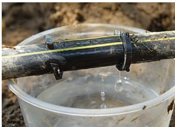
Figure 20. Collecting discharge from a drip emitter.
