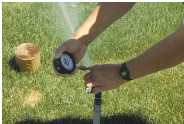
Figure 6. Water pressure is read by positioning the pitot tube directly in the sprinkler's water stream.
