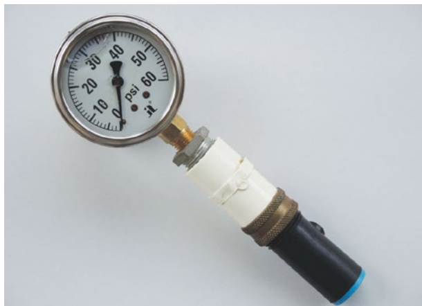
Figure 18. Pressure gauge adapted for measurement at tail end of lateral line microirrigation system tubing. (Photo by L. Schwank)
