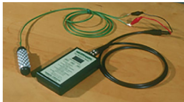
Figure 2. Watermark® soil moisture block and hand reading unit.
