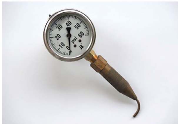
Figure 5. A pitot tube fitted with a pressure gauge works well for taking sprinkler pressure measurements. (Photo by L. Schwankl)
