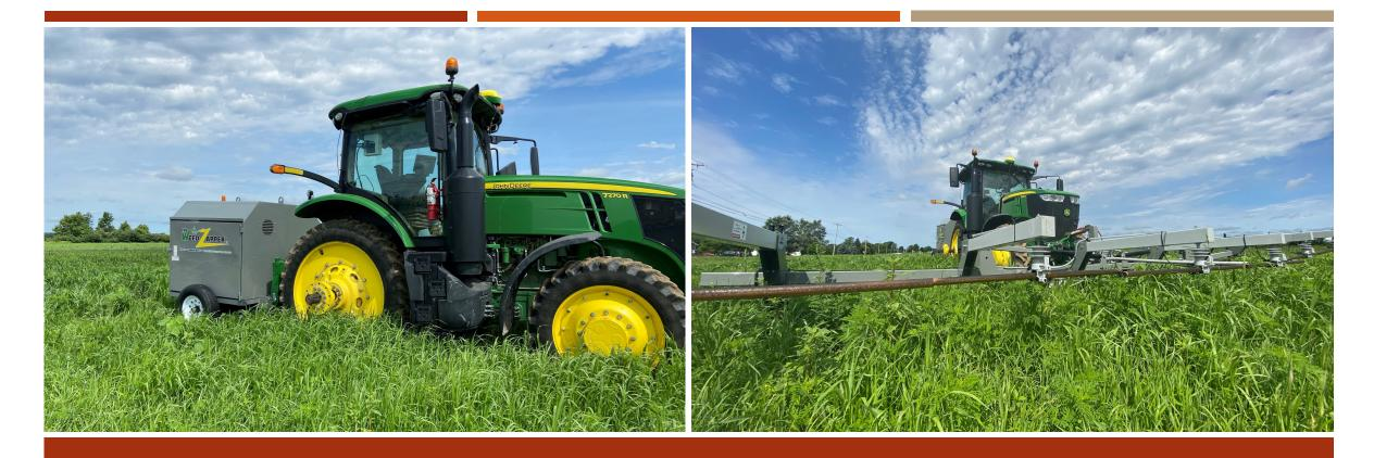
WEED ZAPPER™ IS A TRACTOR-TOWED, PTO-DRIVEN GENERATOR THAT PRODUCES 100,000+ WATTS OF ELECTRICITY THAT CHARGES A FRONT-MOUNTED METAL BAR WEEDS ABOVE THE CANOPY THAT CONTACT THE BAR ARE ELECTROCUTED
